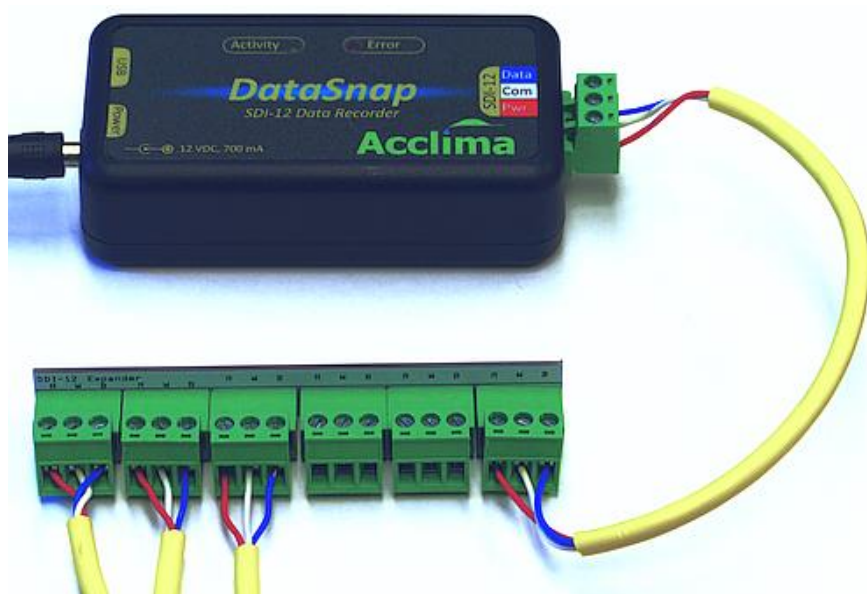
Figure 7 – SDI-12 Port Expander Accessory: Alternative to Splicing
