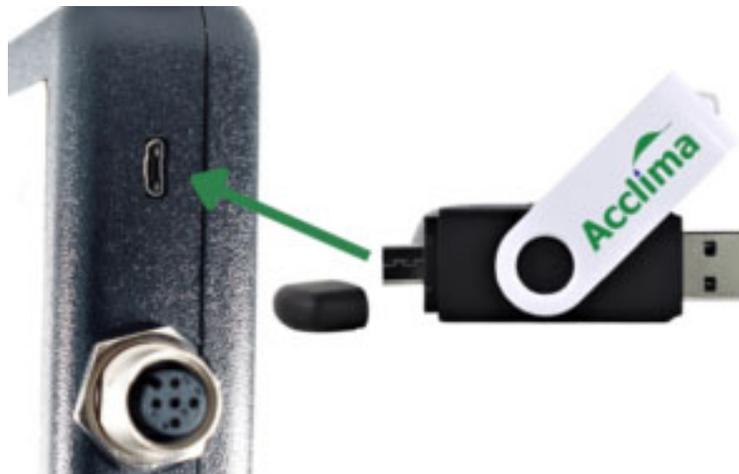
All of the Reader's records will be transferred to the Thumb drive, which can then be connected to your computer's USB port for downloading to the PC and viewing in CSV format. **Important:** Please allow the Reader time to synchronize. Do not disconnect the thumb drive until the Reader indicates the synchronization is complete. It will only take a moment to synchronize.
