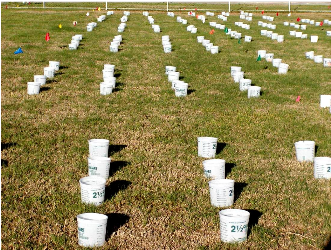
Figure 2-2. Irrigation uniformity distribution test on turfgrass plots.
