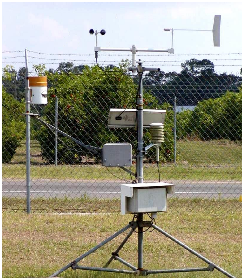
Figure 2-11. Automated weather station near turf plots for this study.
