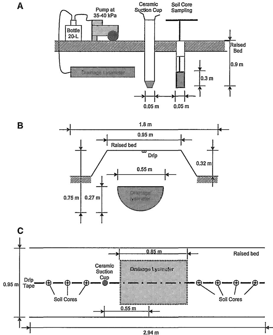
Fig. 2. (A) Overview of instrumentation used for collecting leaching samples, (B) drainage lysimeter layout, and (C) top view of instrumentation distribution.
