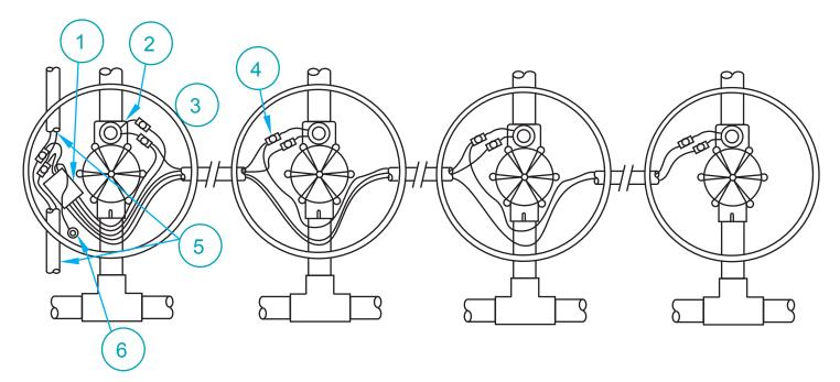
NOTE: MAXIMUM DISTANCE FROM ADAPTER TO SOLENOID VALVE 450'
