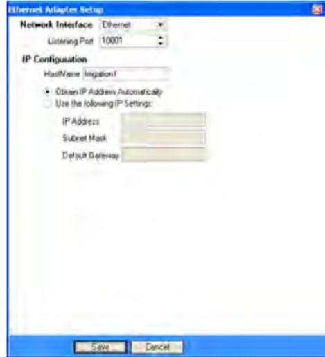
1. Select your desired Network Interface. Choose Ethernet if you are using a CAT-5 wire for communications, or Wireless for 802.11b/g wireless networks.
